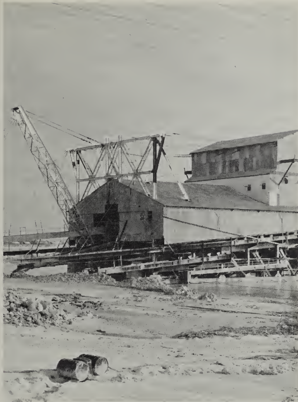
Mining is an important activity in West Malaysia with tin mining of major importance. This tin dredge is at work at a mine just outside Kuala Lumpur.
